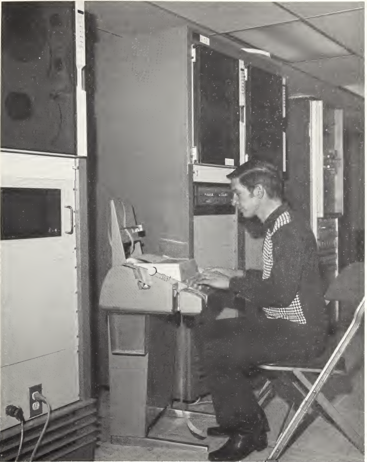
Figure 1-3.--VISSR ingest systems showing tape transports (above), teletype operator interface, GTE minicomputer (at operator eye level), and alpha-numeric display CRT (behind operator and on unit at left)
